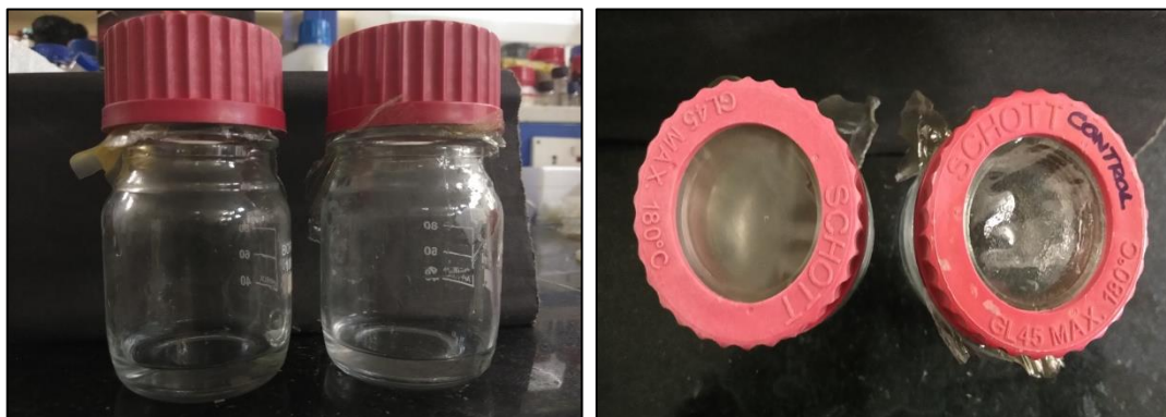
Figure 6.2. Experimental setup for testing the water transfer rate of CS (Control) and CEPSPDO composite films.
