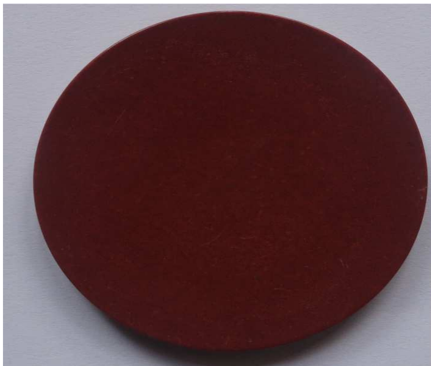
Fig. 5.17 Photograph of 10 wt% Y_2Ce_{1.8}Tb_{0.2}O_7 + PMMA. The polymer matrix exhibit uniform distribution of pigment particles in the substrate.
