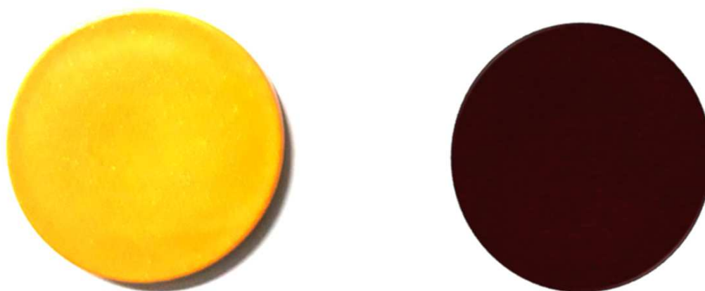
Fig. 6.28 Photograph of 10 wt% SrBaCe_{0.6}Tb_{0.4}O_4 + PMMA and Ba_2Ce_{0.4}Tb_{0.6}O_4 + PMMA. The polymer matrix exhibit uniform distribution of pigment particles in the substrate.
