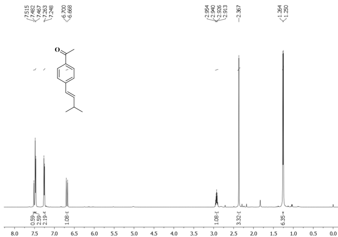
Figure 5B.11: ^1\text{H} NMR spectrum of (E)-1-(4-(3-methylbut-1-en-1-yl) phenyl) ethan-1-one
