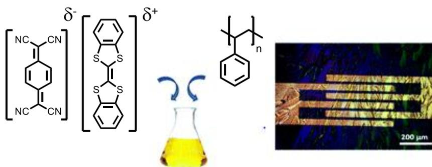
**Figure 1.8.** Ambipolar field effect transistor device fabricated using DBTTF-TCNQ CT complex blended with polystyrene.
