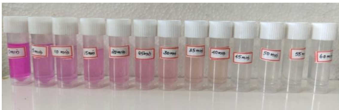
Figure 11. Persulfate activated degradation of RhB on MIL-800 C catalyst.
