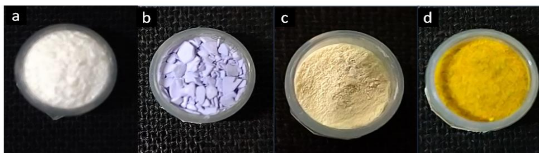
Figure 16. Photographs of a) ZIF-8, b) NiZ, c) NiZC, and d) Ni-methyl imidazolate complex powder samples
