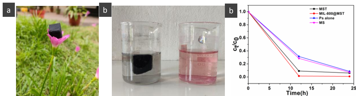
Figure 22. a) The fabrication of MIL-800@MS sponge and b) degradation of RhB at 24 h with and without MIL-800@MST sponge catalyst with [RhB]=30 mg/L and [PS]=5 mM
