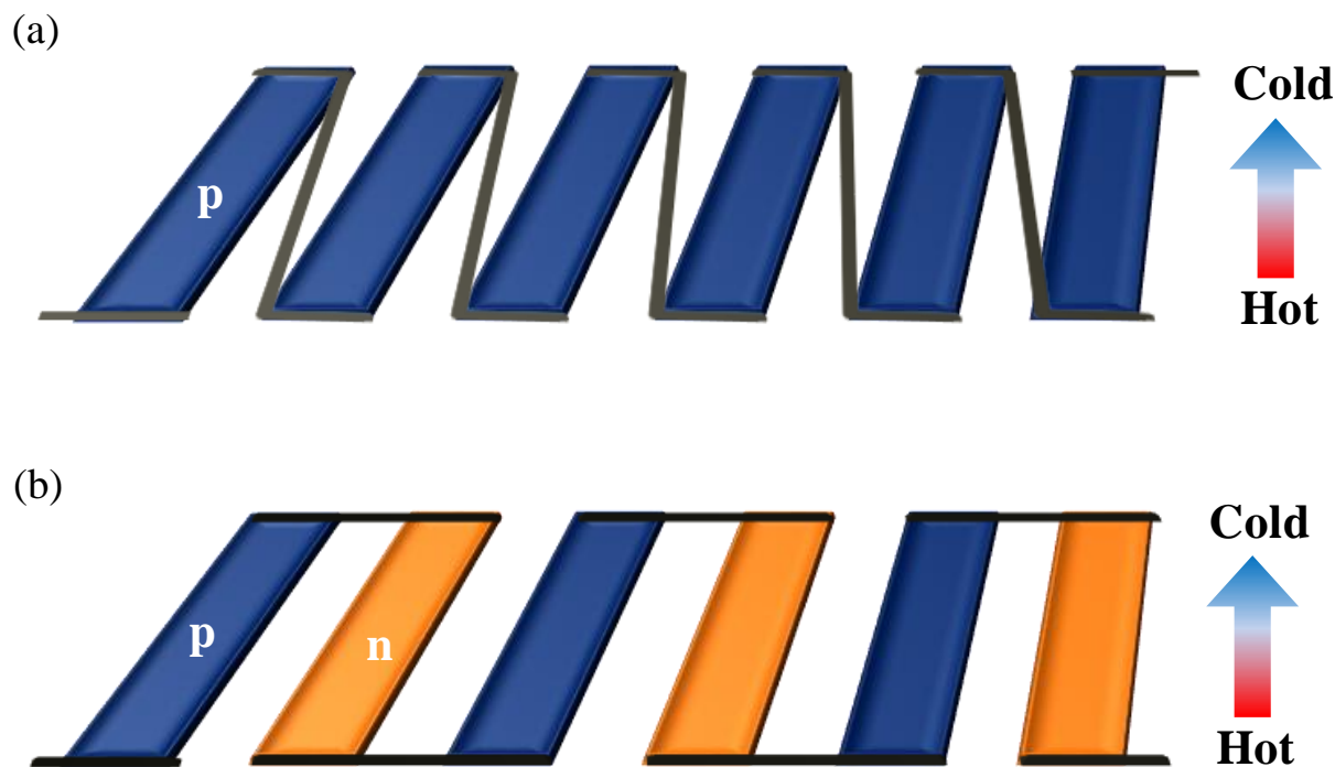
Fig. 1.6. A planar organic TEG with (a) single TE leg and (b) p-n thermocouples. Adapted from Ref. [43].
