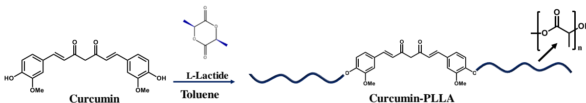
Scheme 4.1. Synthesis of curcumin-embedded PLLA.
