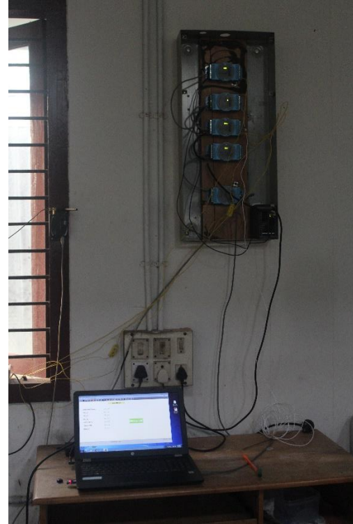
Fig 3.6: Real time recording system with ADAM modules.
