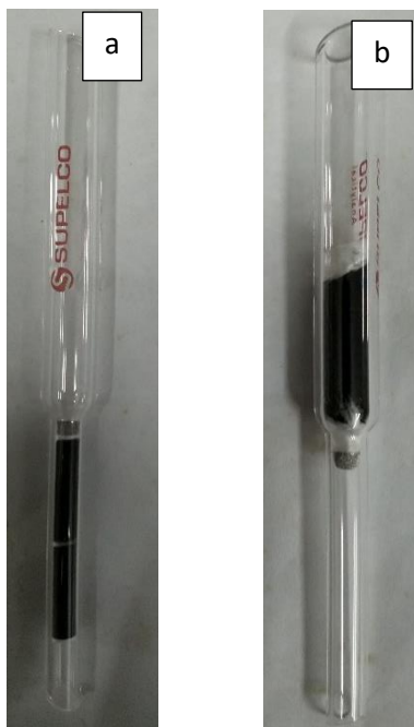
Fig 2.6 a and b: Dual layer carbon column and single layer carbon column respectively.
