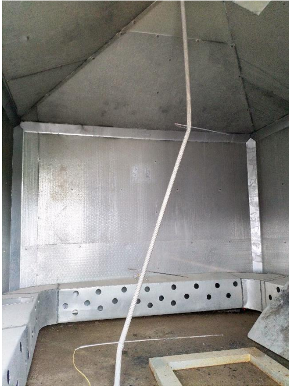
Fig 3.5: Thermocouples in the air pathway to monitor temperature changes.
