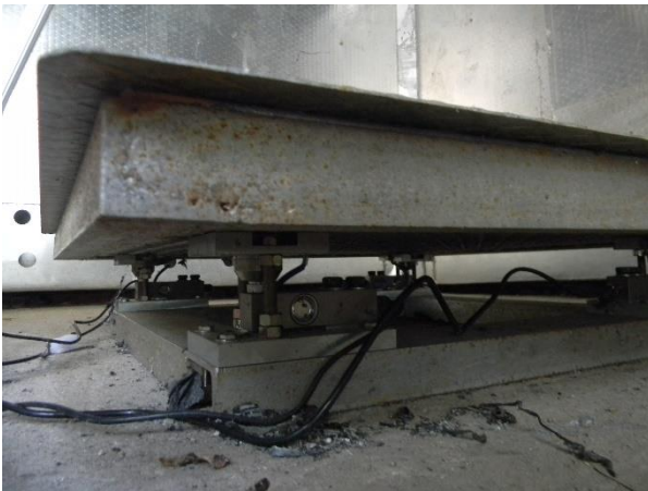
Fig 3.3: Load cell to monitor weight changes.
