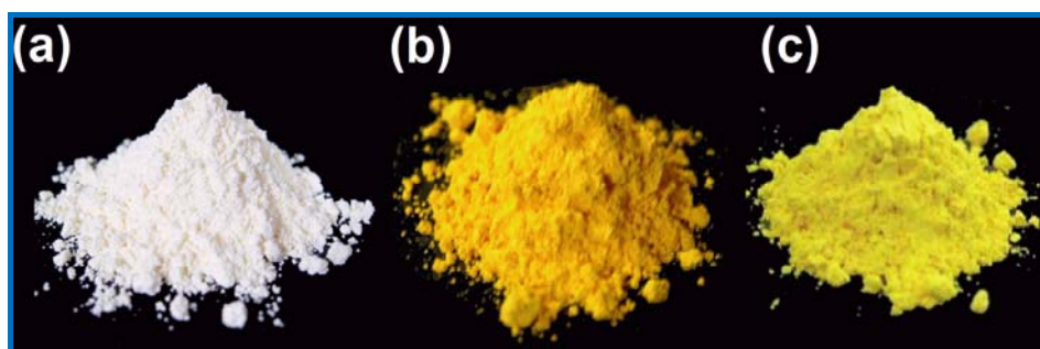
Fig. 1.15. Photographs of (a) Ce_{0.43}Zr_{0.37}La_{0.20}O_{1.9} , (b) Ce_{0.43}Zr_{0.37}Bi_{0.20}O_{1.9} and (c) praseodymium yellow.
